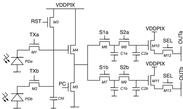
**Figure 1: Circuit diagram of the 2x1 shared global shutter pixel**
