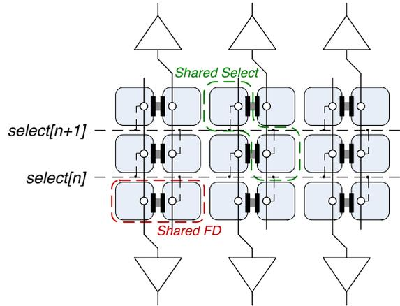
**Figure 2: Schematic view on pixel sharing for charge sensing and readout**
