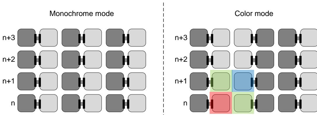
**Figure 4: Integration shift implementation for monochrome and color mode operation.**
