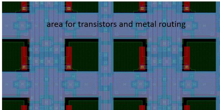
**Figure 5: Global shutter pixel layout at 3.5  $\mu\text{m}$  pitch.**
