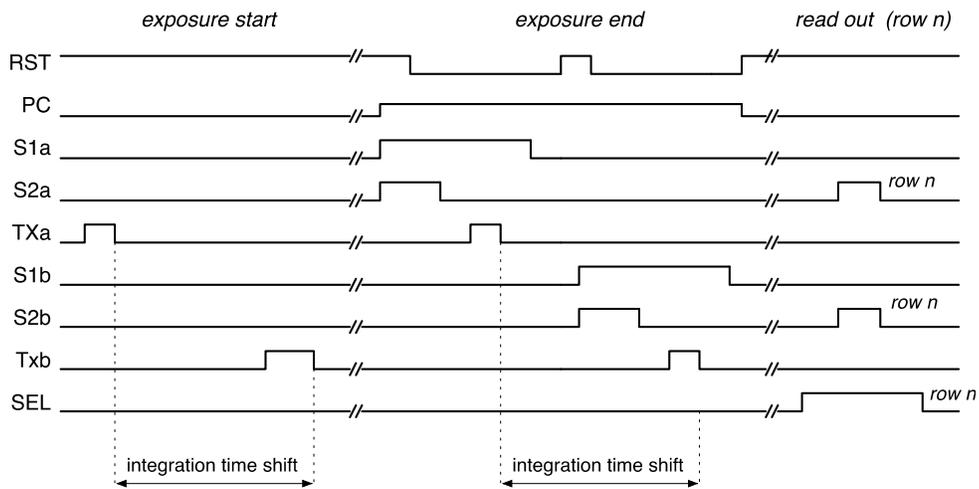
**Figure 3: Pixel timing for start and end of exposure and during readout**
